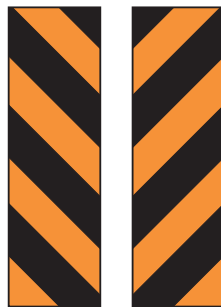
Hazard to left Hazard to right
